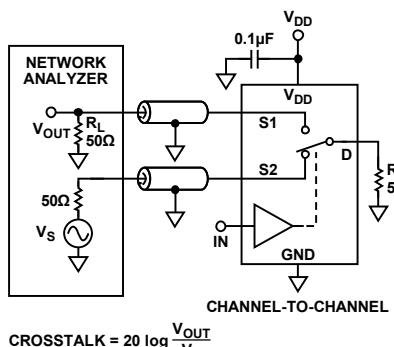
Figure 19. Channel-to-Channel Crosstalk
