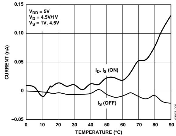
Figure 6. Leakage Currents vs. Temperature
