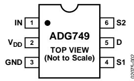
Figure 2. Pin Configuration
