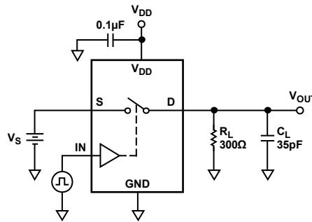
Figure 16. Switching Times
