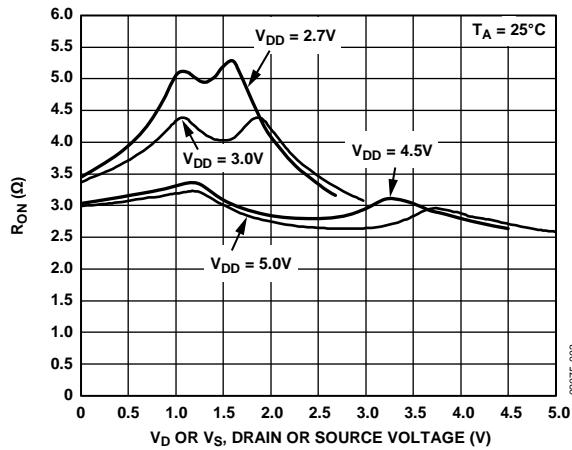
Figure 3. On Resistance vs.  $V_D$  ( $V_S$ ) Single Supplies
