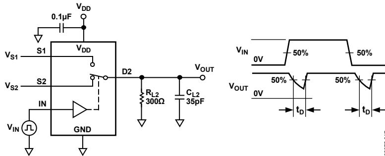
Figure 17. Break-Before-Make Time Delay,  $t_D$
