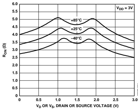
Figure 4. On Resistance vs.  $V_D$  ( $V_S$ ) for Different Temperature,  $V_{DD} = 3\text{ V}$
