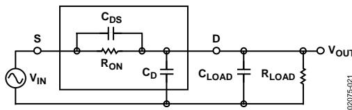
Figure 21. Switch Represented by Equivalent Parasitic Components
