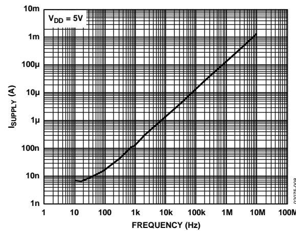
Figure 8. Supply Current vs. Input Switching Frequency
