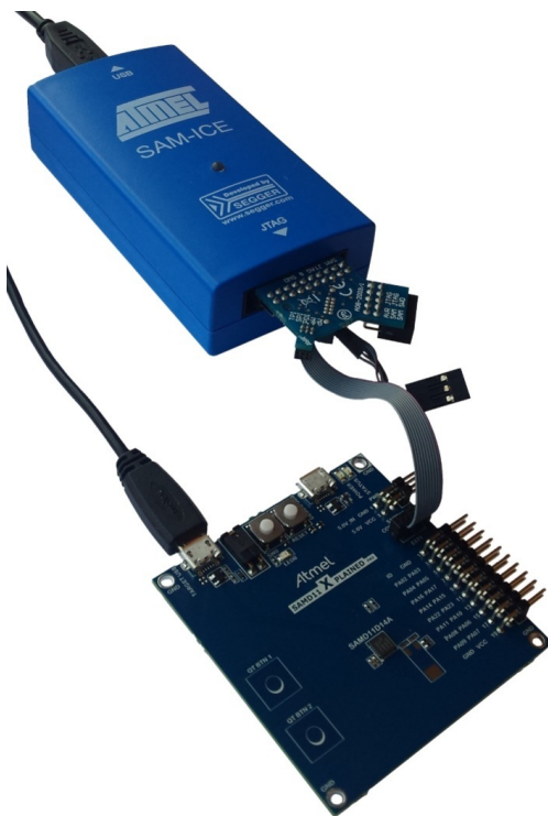
Figure 5-7. SAM-ICE using an Atmel-ICE Adapter
