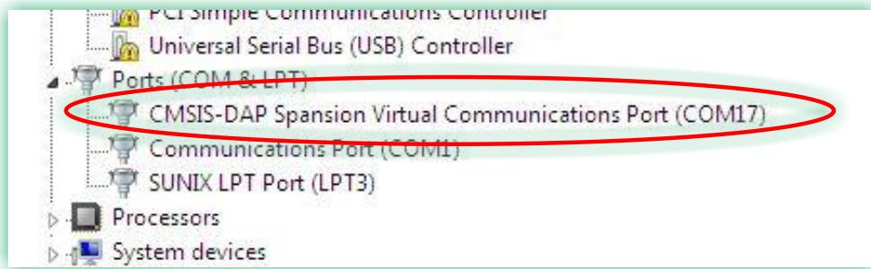
**Figure 5: WyzBee™ CMSIS-DAP Debug Port Detection**
