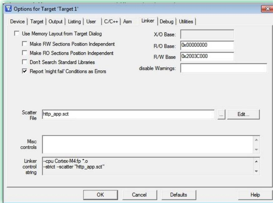
**Figure 13: Keil uVision: Options for Target – Linker**
