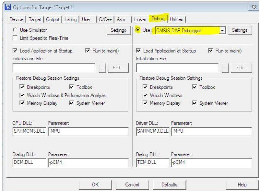
**Figure 9: Keil uVision: Options for Target – Debug**
