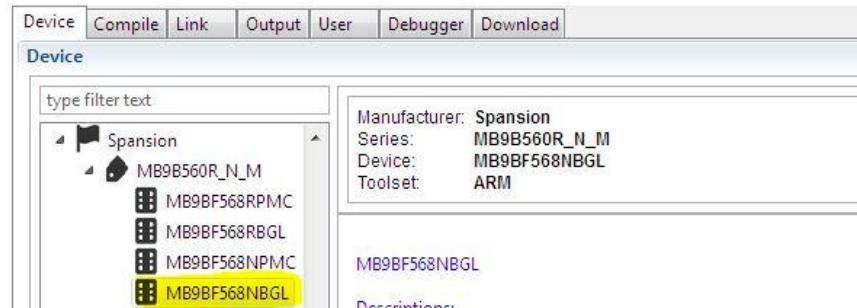
**Figure 30: CoIDE Configuration – Device**
