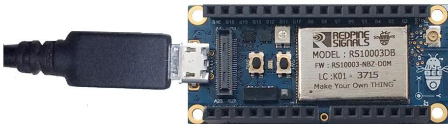
Figure 1: WyzBee™ Baseboard with micro-B USB Cable
