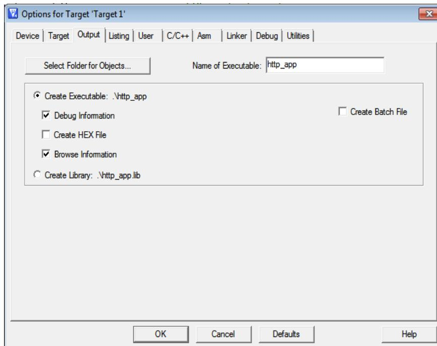
**Figure 12: Keil uVision: Options for Target – Output**
