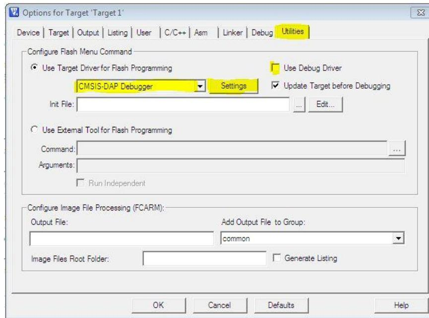
**Figure 7: Keil uVision: Options for Target – Utilities**
