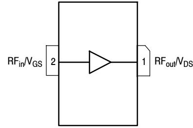
**Figure 1. Pin Connections**
