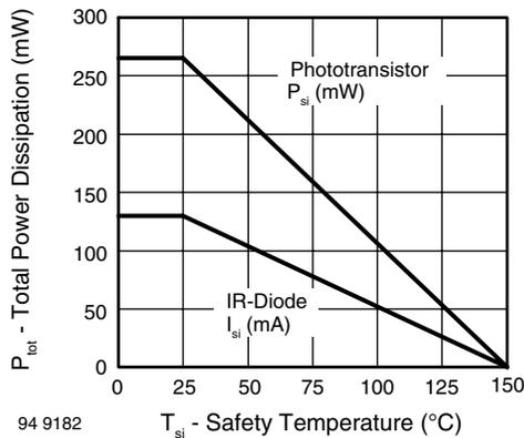
Fig. 1 - Derating Diagram
