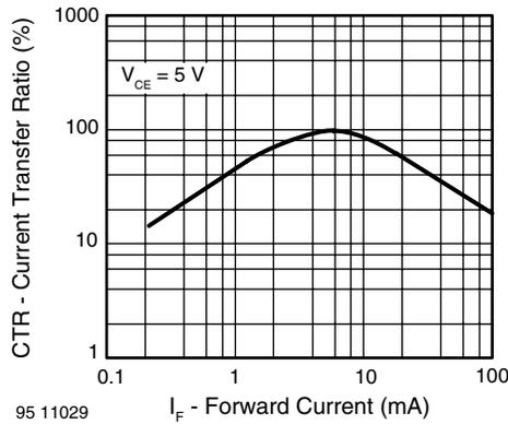
Fig. 13 - Current Transfer Ratio vs. Forward Current
