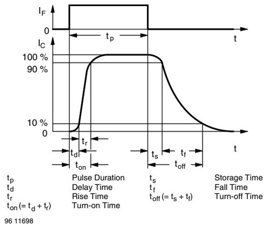
Fig. 5 - Switching Times
