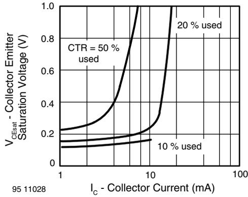
Fig. 12 - Collector Emitter Saturation Voltage vs. Collector Current
