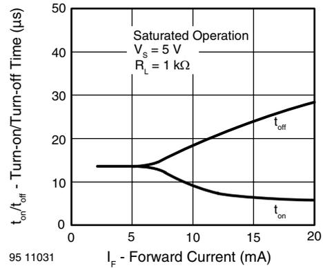
Fig. 15 - Turn-on/off Time vs. Forward Current
