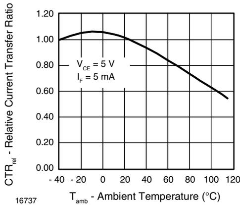
Fig. 8 - Relative Current Transfer Ratio vs. Ambient Temperature
