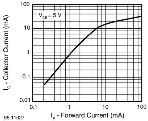
Fig. 10 - Collector Current vs. Forward Current
