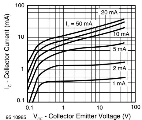
Fig. 11 - Collector Current vs. Collector Emitter Voltage
