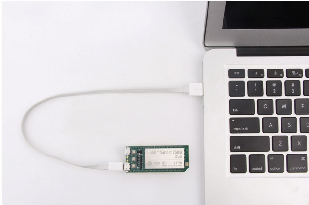
Figure 14 Connecting LinkIt Smart development board to a computer
