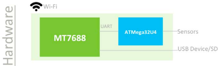
Figure 52 Smart 7688 Duo Hardware Architecture
