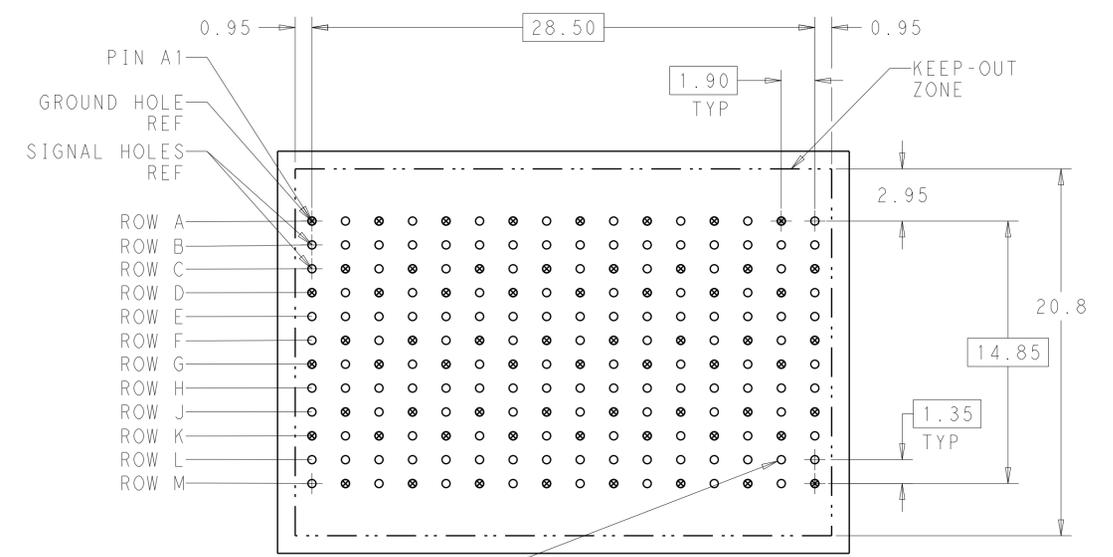
192X  $\varnothing 0.46 \pm 0.05$  PLATED THRU HOLE
