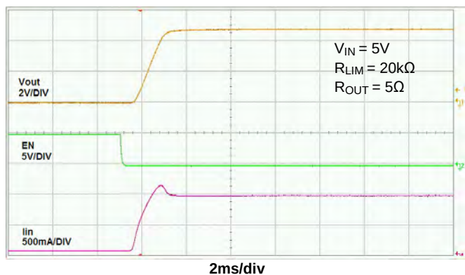
Figure 3. Turn-On Delay and Rise Time
