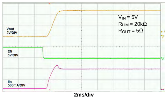
Figure 3. Turn-On Delay and Rise Time
