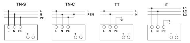
The 100 V AC ... 240 V AC connection is made using the L and N screw connections.
