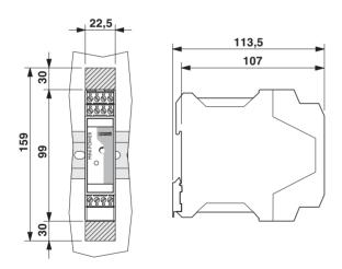
Installation: Installation depth 95 mm (+ DIN rail)
