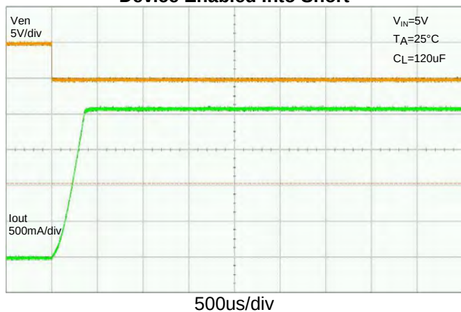
Short Circuit Current, Device Enabled Into Short
