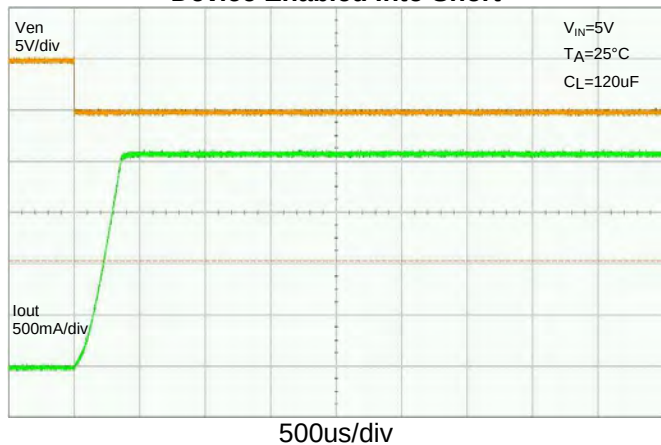
Short Circuit Current, Device Enabled Into Short
