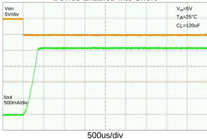
Short Circuit Current, Device Enabled Into Short
