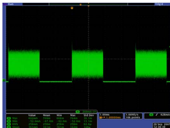
FIGURE 11. I_L AT 50% PWM DIMMING
