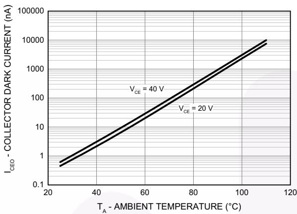
Figure 9. Collector Dark Current vs. Ambient Temperature
