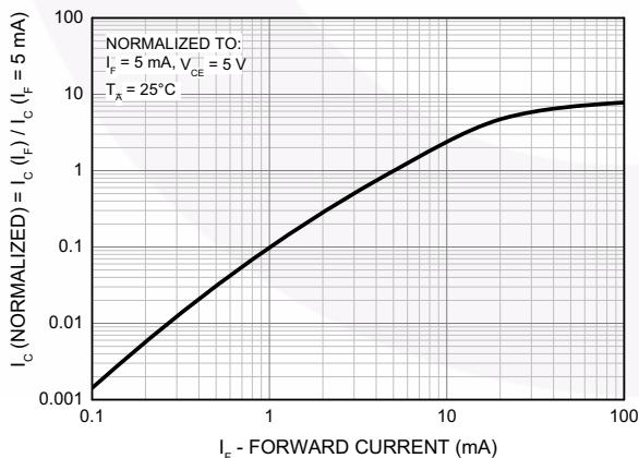
Figure 7. Normalized Current Collector vs. Forward Current
