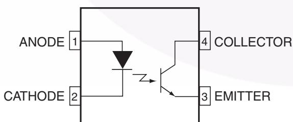
Figure 1. Schematic
