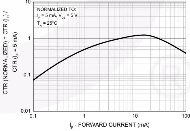
Figure 8. Normalized Current Transfer Ratio vs. Forward Current
