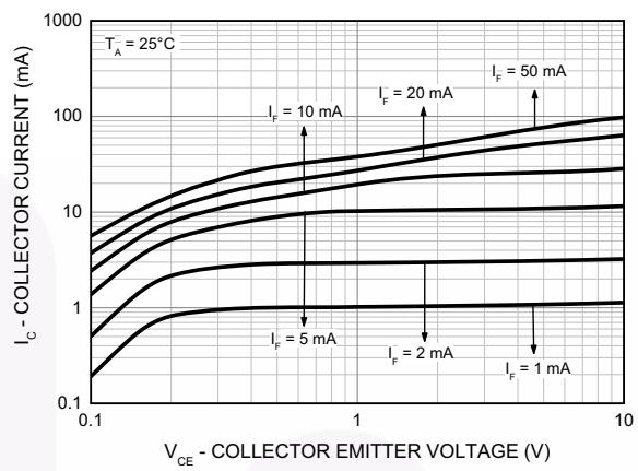
Figure 10. Collector Current vs. Collector Emitter Voltage
