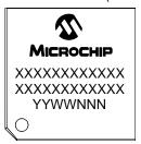
100-Lead TQFP (12x12x1 mm)
