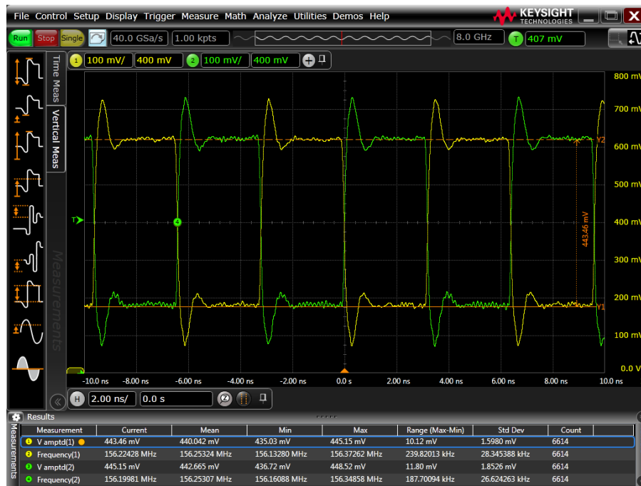
Figure 5-1. LVPECL 3.3 V, 156.25 MHz Clock Measured with DC Coupling, 50-Ω Scope Termination
