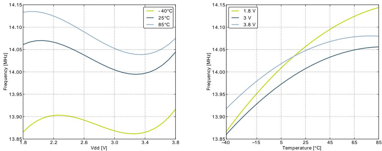
**Figure 3.23. Calibrated HFRCO 21 MHz Band Frequency vs Supply Voltage and Temperature**
