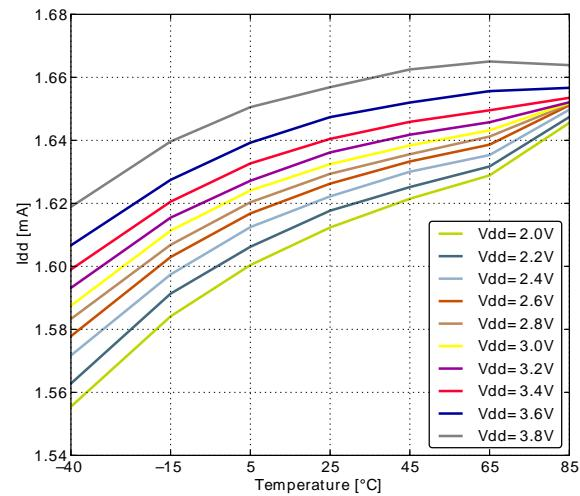
**Figure 3.4. EMO Current consumption while executing prime number calculation code from flash with HFRCO running at 11MHz**
