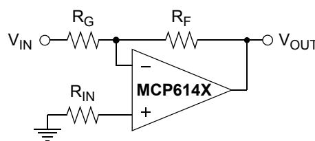
**FIGURE 4-4:** Noise Gain for Inverting Gain Configuration.
