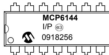
14-Lead SOIC (150 mil) (**MCP6144**)
