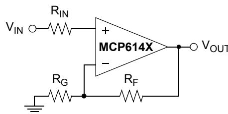
**FIGURE 4-3:** Noise Gain for Non-inverting Gain Configuration.
