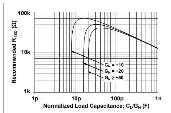
**FIGURE 4-7:** Recommended  $R_{ISO}$  Values for Capacitive Loads.
