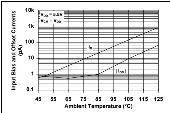
**FIGURE 2-13:** Input Bias, Offset Currents vs. Ambient Temperature.
