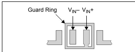
FIGURE 4-9: Example Guard Ring Layout for Inverting Gain.
