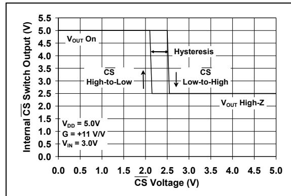
**FIGURE 2-35:** Internal Chip Select ( $\overline{\text{CS}}$ ) Hysteresis (MCP6143 only).
