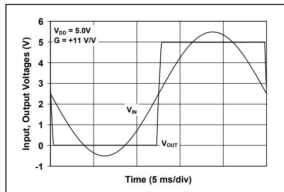
**FIGURE 2-10:** The MCP6141/2/3/4 Family Shows No Phase Reversal.
