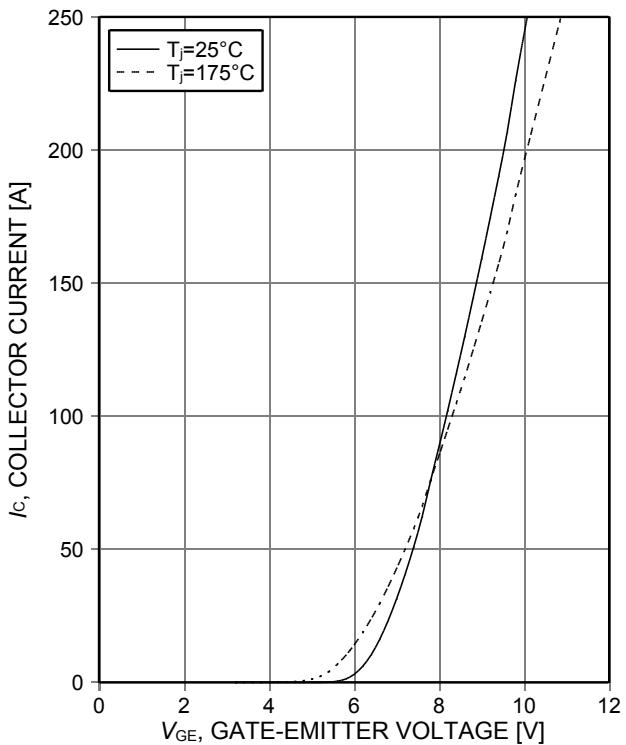
Figure 7. **Typical transfer characteristic**
