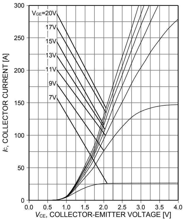
Figure 5. **Typical output characteristic**
