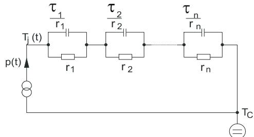
Figure D. Thermal equivalent circuit
