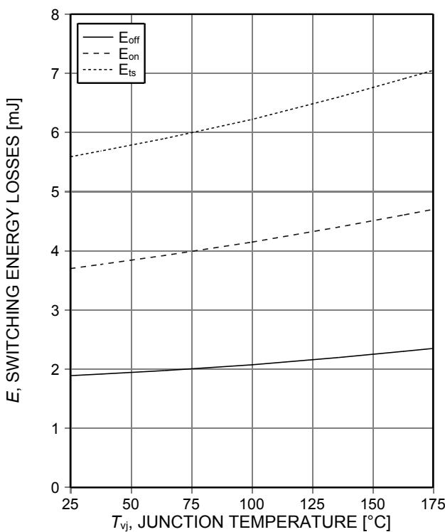
Figure 15. **Typical switching energy losses as a function of junction temperature**
