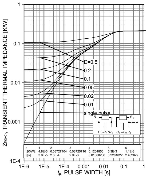
Figure 21. IGBT transient thermal impedance
