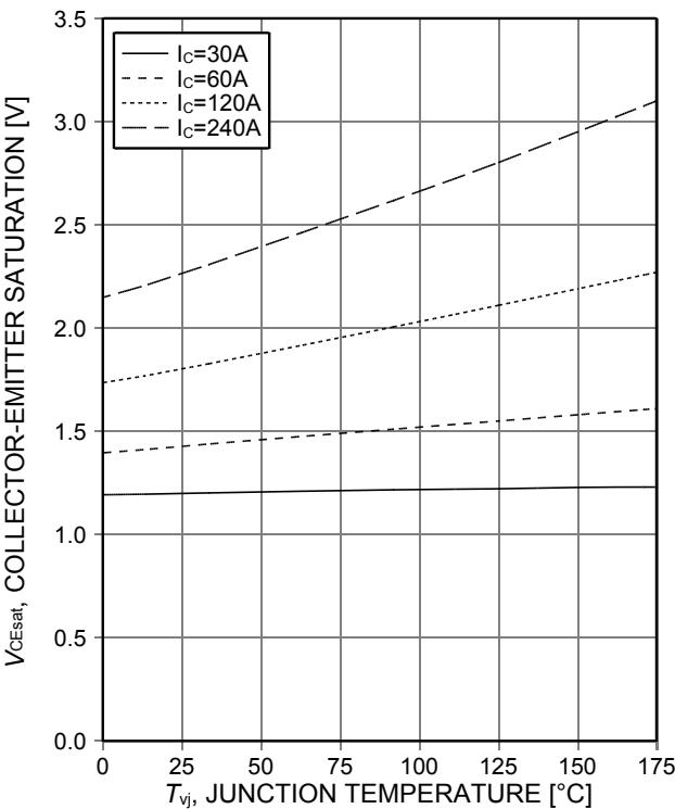
Figure 8. **Typical collector-emitter saturation voltage as a function of junction temperature**
