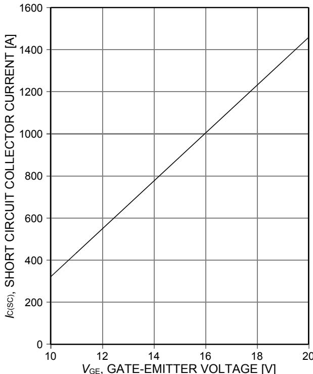
Figure 19. Typical short circuit collector current as a function of gate-emitter voltage
