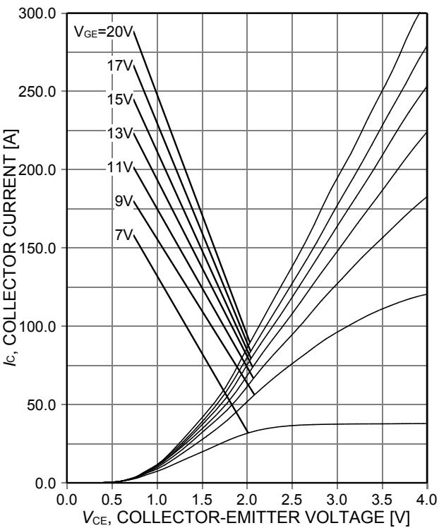
Figure 6. **Typical output characteristic**
