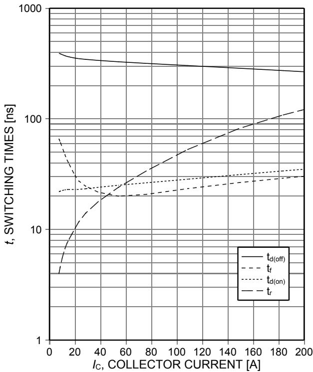
Figure 9. Typical switching times as a function of collector current
