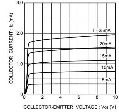
Fig.10 Output characteristics
