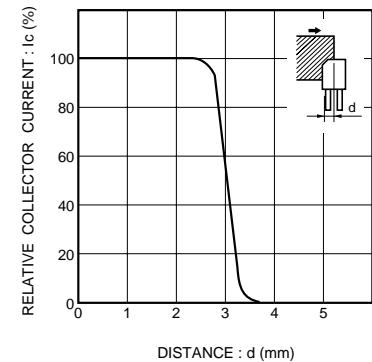
Fig.1 Relative output vs. distance (I)
