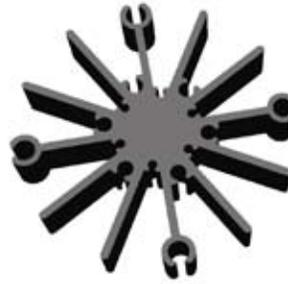
Ohmite S Series LED Heatsinks are low cost and easy assembly heat sinks for "Star" LED packages supplied by Cree, Lumileds, Osram and others. This simple heat sink can hold LED modules and can be mounted simply with some thread forming screws. The heat sink has two types of surface finish and can be used in either natural (free) or forced convection cooling applications.
