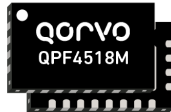
24 Pin 5x3 mm QFN Package
