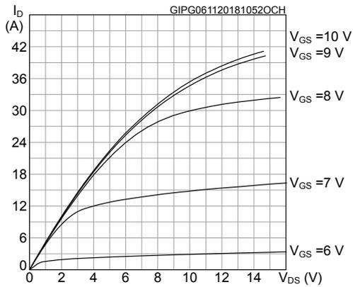
Figure 4. Transfer characteristics
