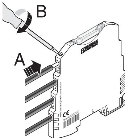
Figure 5 Screw connection
