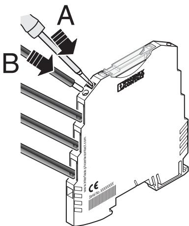
Figure 3 Spring-cage connection
