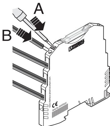
Figure 6 Spring-cage connection
