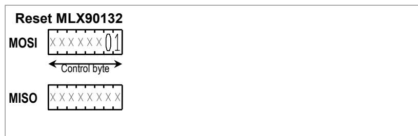
Figure 9: SPI communication reset the MLX90132
