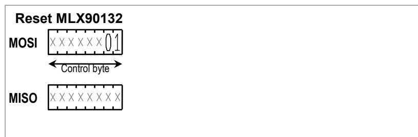
Figure 9: SPI communication reset the MLX90132
