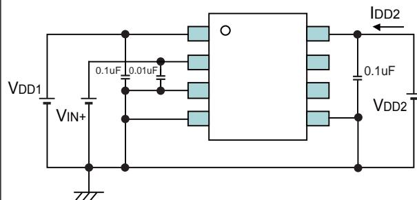
Fig.3 IIN Test Circuit
