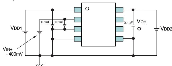
Fig.5 Iosc Test Circuit
