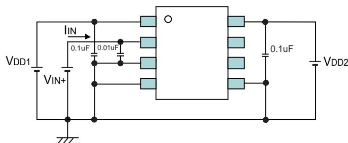
Fig.4 Vout Test Circuit
