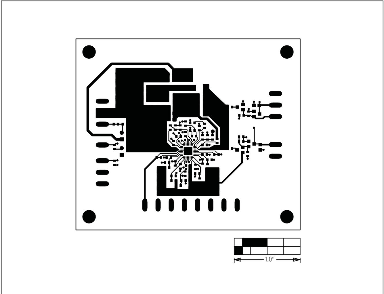
Figure 3. MAX8795A EV Kit PCB Layout—Component Side
