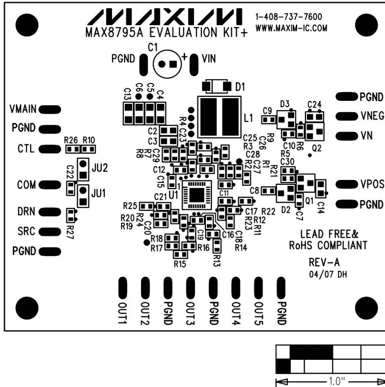
Figure 2. MAX8795A EV Kit Component Placement Guide—Component Side
