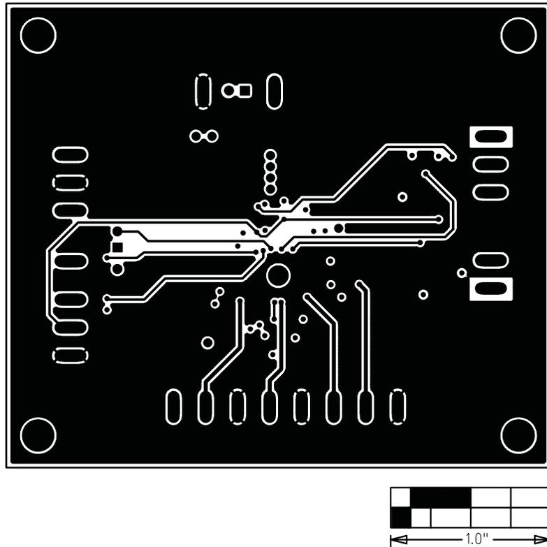
Figure 5. MAX8795A EV Kit PCB Layout—Internal Layer 3 (Signal/GND Plane)
