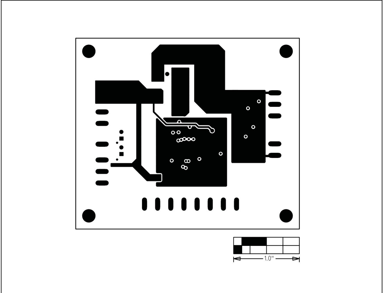
Figure 6. MAX8795A EV Kit PCB Layout—Solder Side
