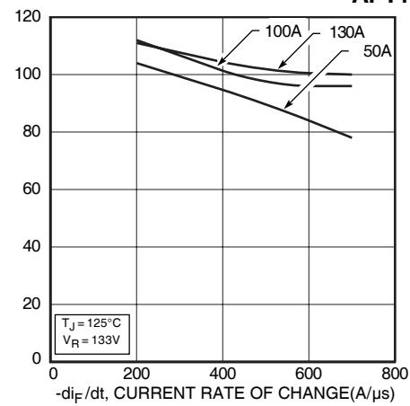
Figure 3. Reverse Recovery Time vs. Current Rate of Change
