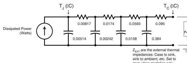
FIGURE 1b. TRANSIENT THERMAL IMPEDANCE MODEL
