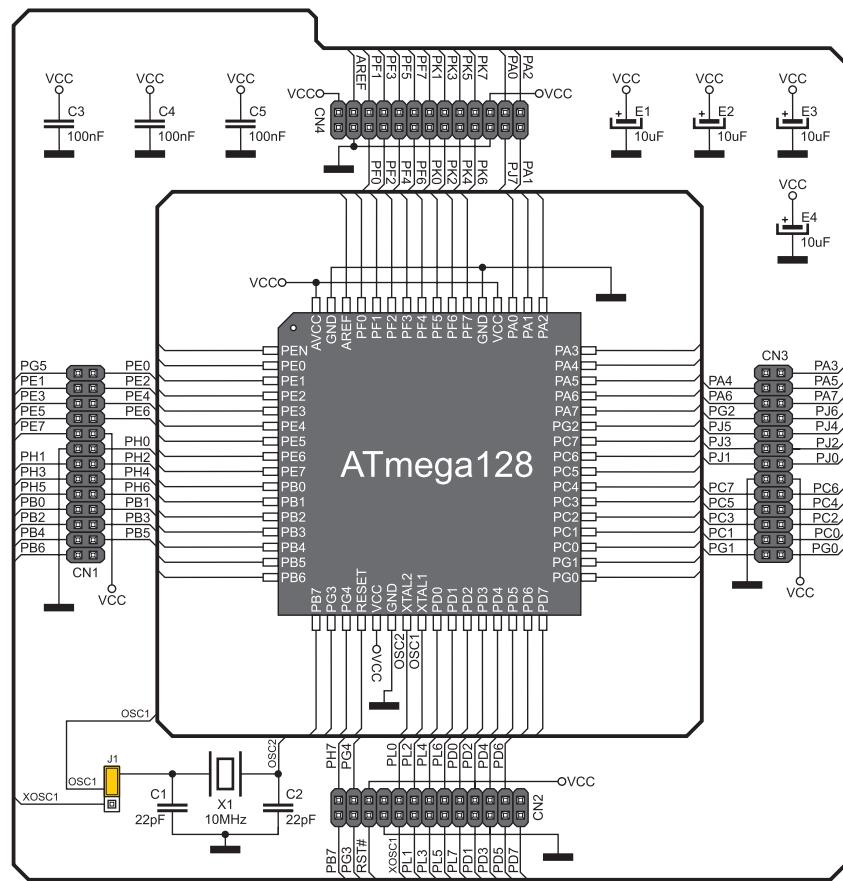
Figure 1: 64-pin MCU card and microcontroller connection schematic
