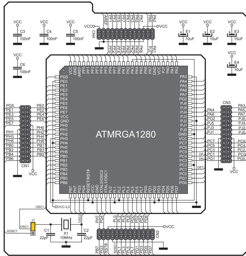
Figure 2: 100-pin MCU card and microcontroller connection schematic
