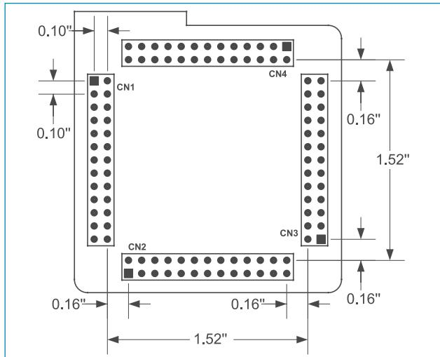
Figure 1-4: Dimensions of MCU card for BIGAVR2
