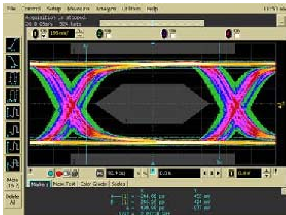
Figure 5: 8bit deep color DVI/HDMI TX eye tested with 20 meter. 24 AWG HDMI cable. Setting: Optimized equalization, 0dB output pre-emphasis and de-emphasis, and Swing 500mV.
