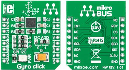
Gyro Click™ is an accessory board in mikroBUS™ form factor. It's a compact and easy solution for adding gyroscope to your design. It features **L3GD20** three-axis digital gyroscope module. Gyro Click™ communicates with the target board microcontroller via mikroBUS™ SPI (MOSI, MISO, SCK, CS), I<sup>2</sup>C (SDA, SCL), INT and RST lines. The board is designed to use 3.3V power supply only. LED diode (GREEN) indicates the presence of power supply.
