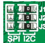
The Gyro Click™ board communicates with the main board microcontroller via I<sup>2</sup>C or SPI interface depending on the position of the **J1**, **J2** and **J3** SMD jumpers. These jumpers are soldered in I<sup>2</sup>C interface position by default. There is an option to select the alternate address with jumper **J4** in the case of I<sup>2</sup>C interface (default position is logic 1).
