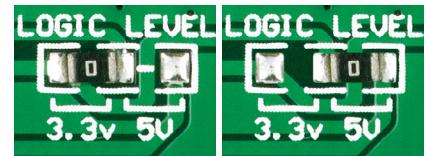
To switch between 3.3V and 5V power supplies, use the on-board zero-ohm SMD jumper. By default it's soldered in the 3.3V position.
