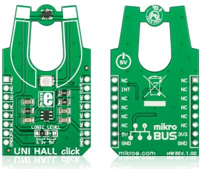
UNI HALL click™ is a simple solution for adding an unipolar Hall switch to your design. It carries the Melexis US5881 unipolar Hall-effect switch and a 74LVC1T45 single bit, dual supply translating transceiver. UNI HALL click™ communicates with the target board through the mikroBUS™ INT line. The board is designed to use either a 3.3V or 5V power supply (which also defines the logic level of the output signal).
