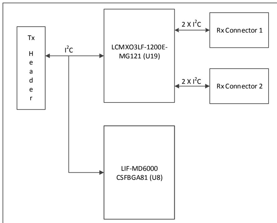
Figure 3.3. I<sup>2</sup>C Expander Block
