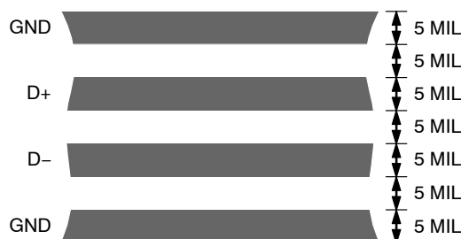
Figure 34. Typical Arrangement of Signal Tracks
