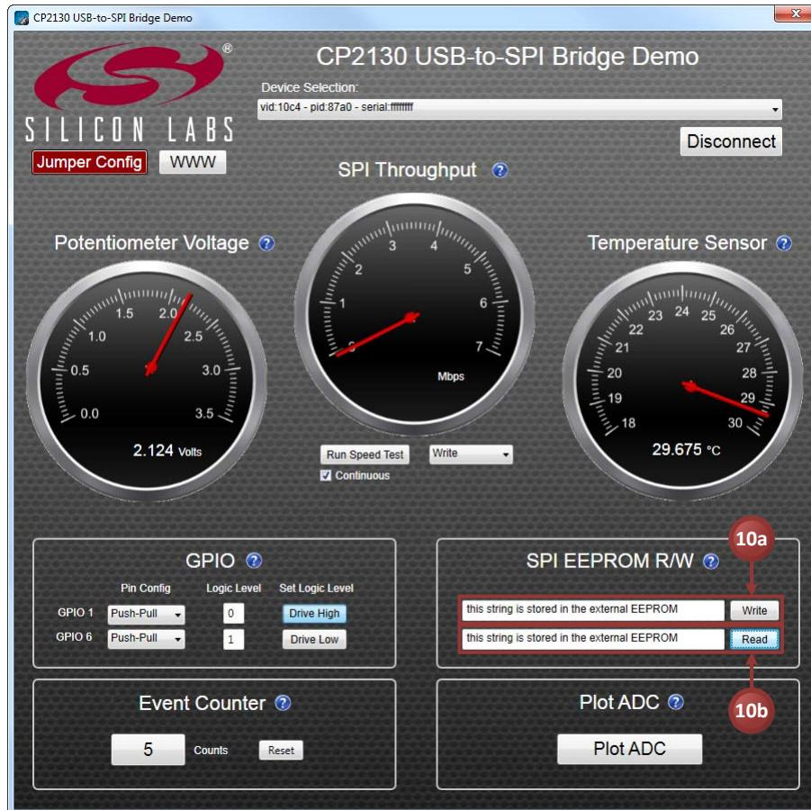
Figure 8. Reading and Writing the SPI EEPROM
