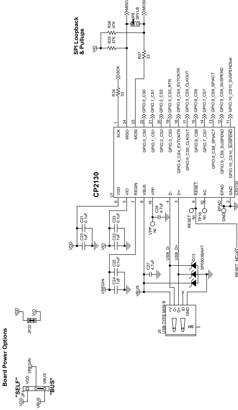
Figure 20. CP2130 Evaluation Board Schematic (1 of 2)
