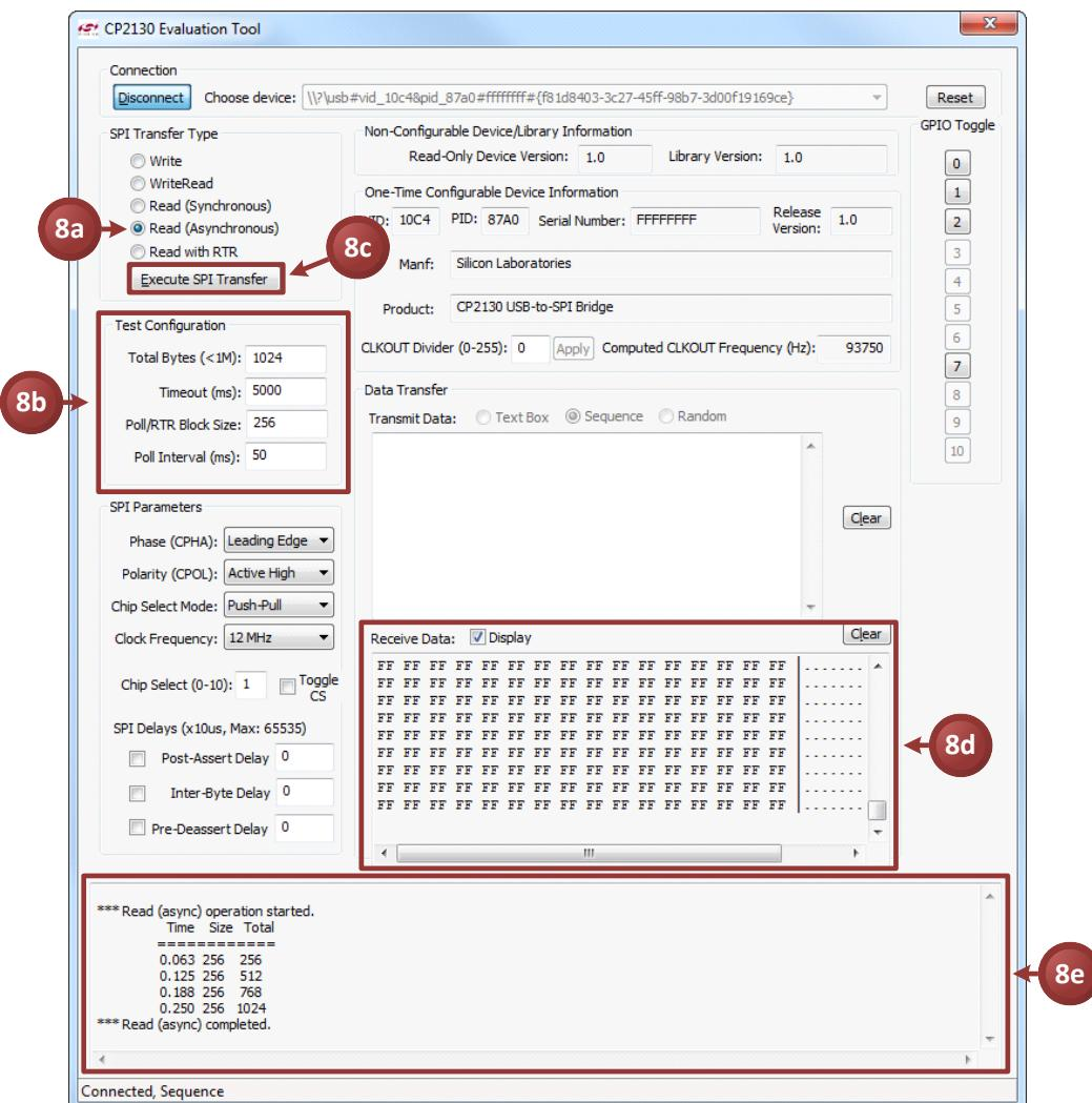
Figure 15. Executing an Asynchronous Read SPI Transfer
