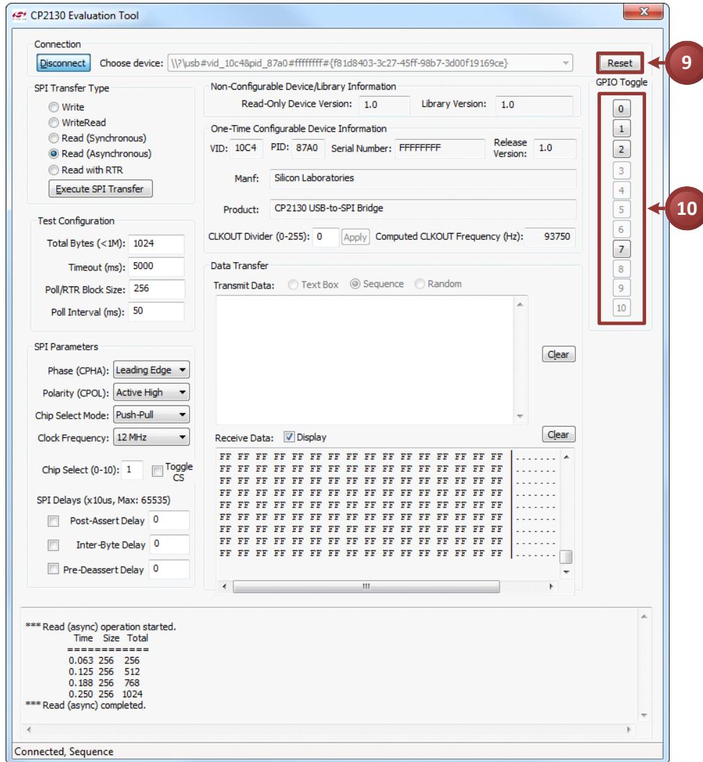
**Figure 16. Resetting the Device and Toggling GPIO Pins**
