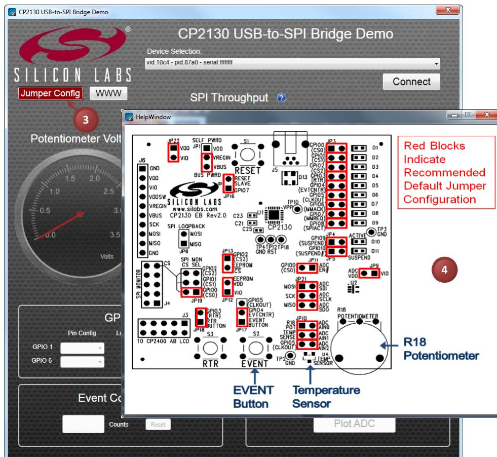
**Figure 3. Configuring the CP2130 Evaluation Board Shorting Blocks**
