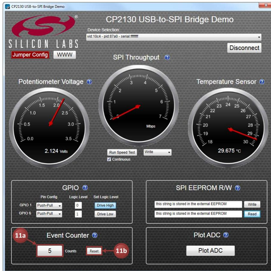
Figure 9. Monitoring Push-Button Presses Using the Event Counter
