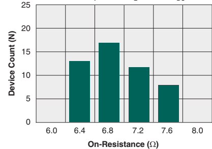
Typical On-Resistance Distribution (N=50, I_F=5mA , I_L=170mA_{DC} )
