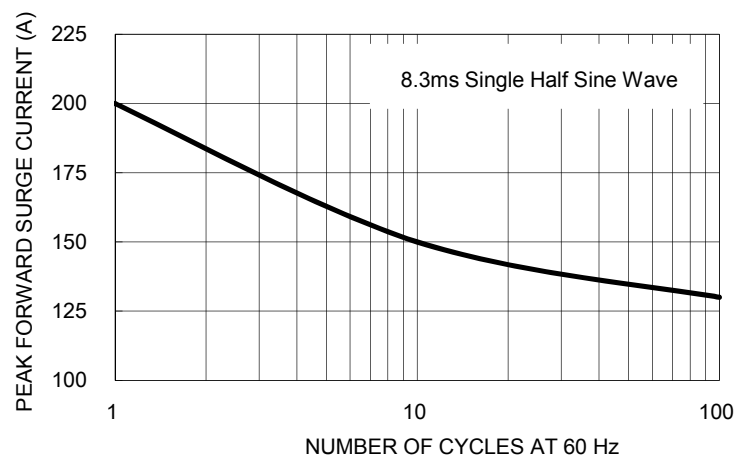
FIG. 2 MAXIMUM NON-REPETITIVE FORWARD SURGE CURRENT PER LEG
