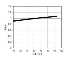
Fig.8 IOUT Temperature dependency ( 100 lx )
