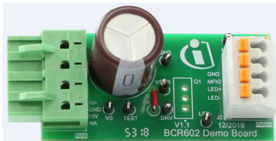
Figure 2 Top side of the demonstrator design board (56.00 mm x 27.00 mm)
