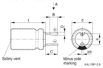
The series B41897 and B41898 have no sleeve nor minus pole marking, the positive pole is marked on the aluminum case side instead.
