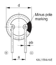
The series B41897 and B41898 have no sleeve nor minus pole marking, the positive pole is marked on the aluminum case side instead.
