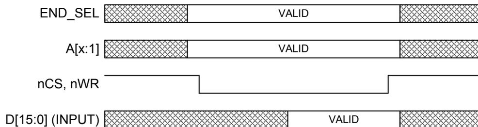
**Figure 8.7 Functional Timing for PIO Write Operation**
