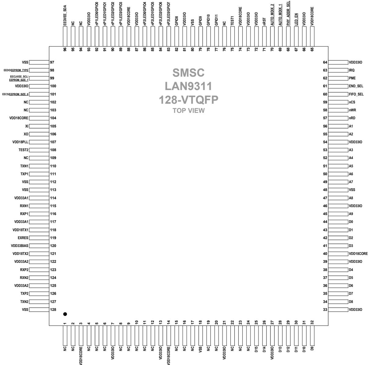
Figure 3.1 LAN9311 128-VTQFP Pin Assignments (TOP VIEW)
