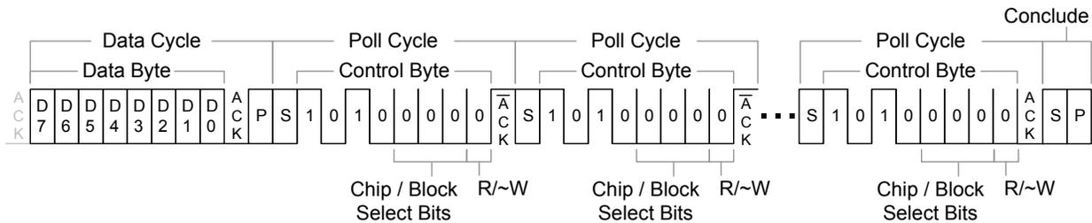
**Figure 10.6 I<sup>2</sup>C EEPROM Byte Write**
