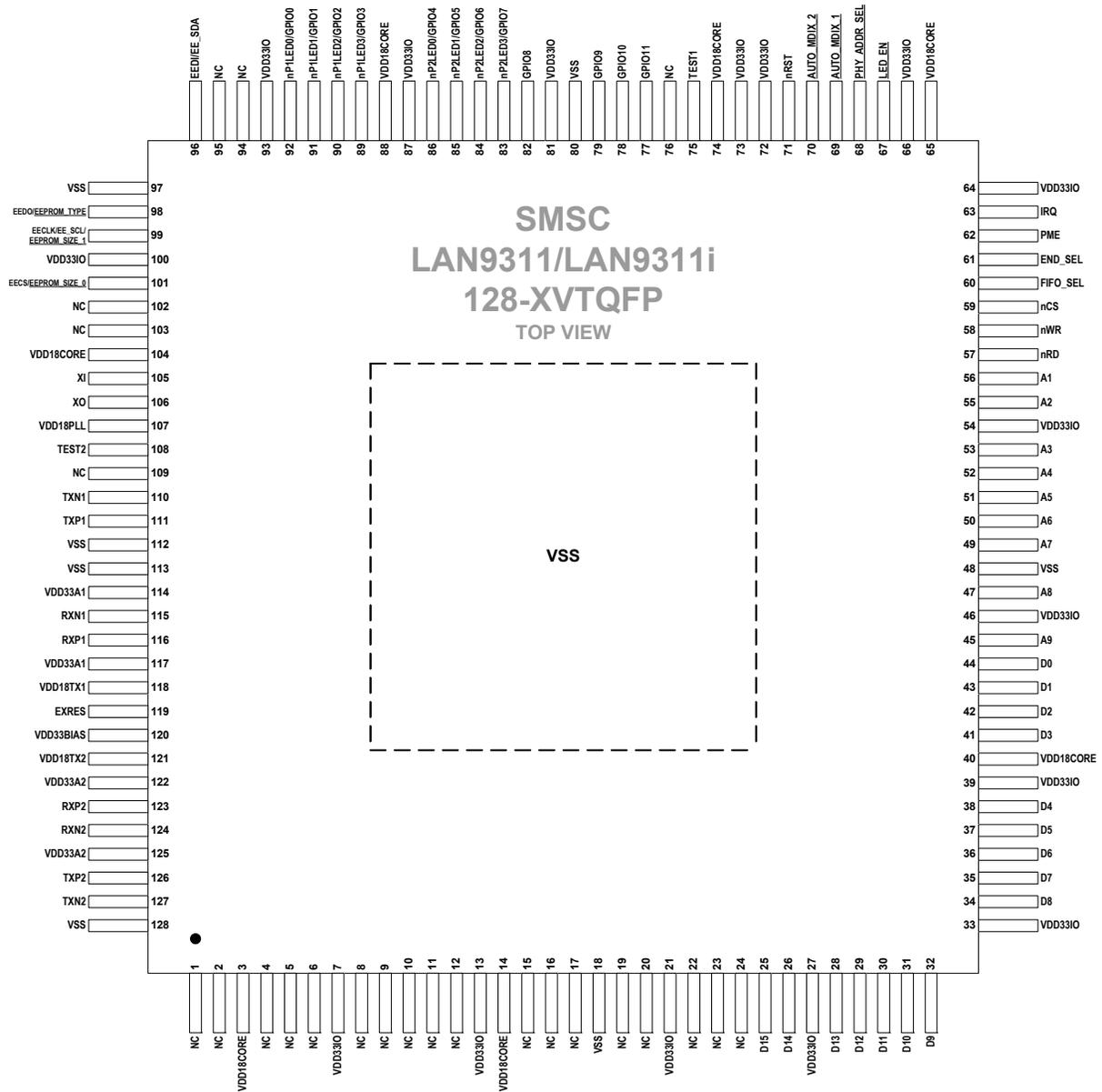
NOTE: EXPOSED PAD ON BOTTOM OF PACKAGE MUST BE CONNECTED TO GROUND
