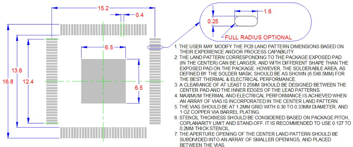
**Figure 16.4 LAN9311/LAN9311i 128-XVTQFP Recommended PCB Land Pattern**
