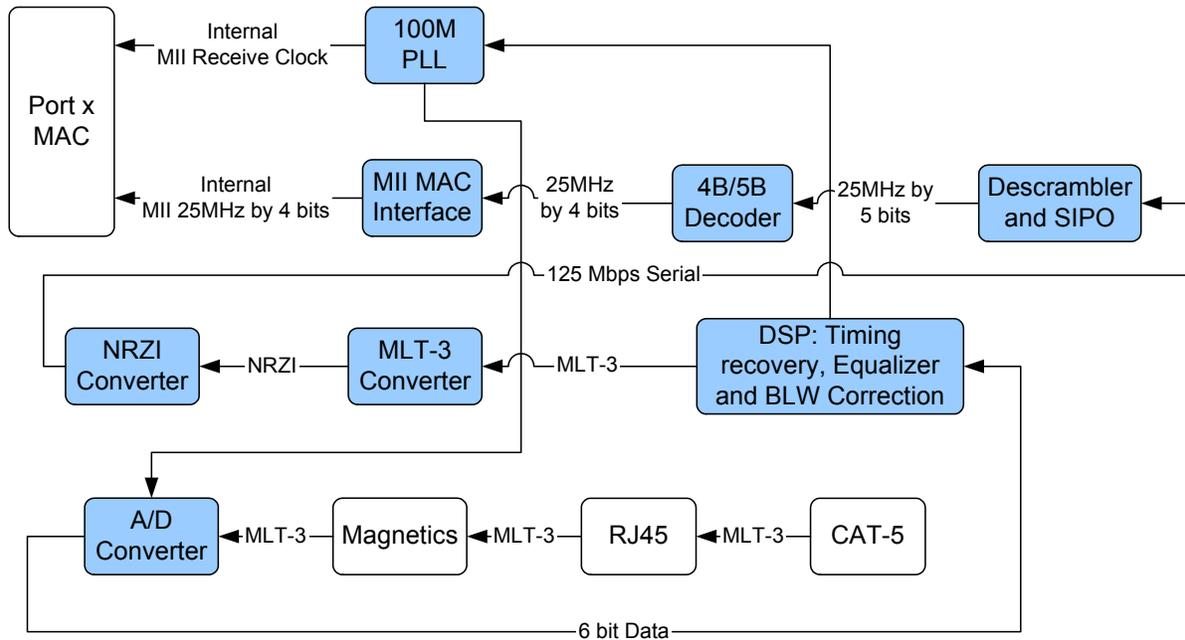
Figure 7.3 100BASE-TX Receive Data Path
