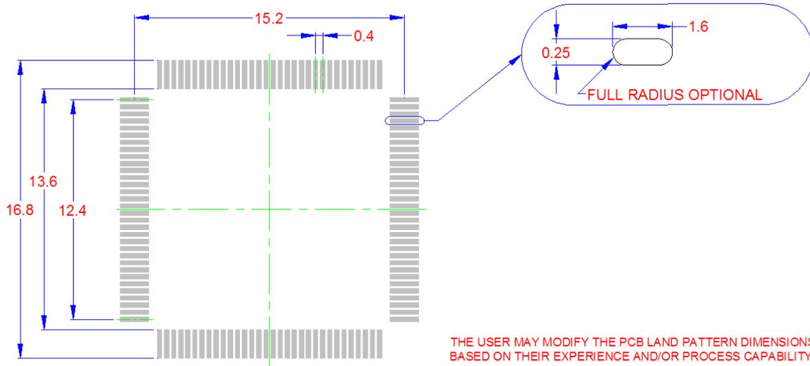
**Figure 16.2 LAN9311 128-VTQFP Recommended PCB Land Pattern**
