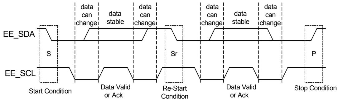
**Figure 10.2 I<sup>2</sup>C Cycle**
