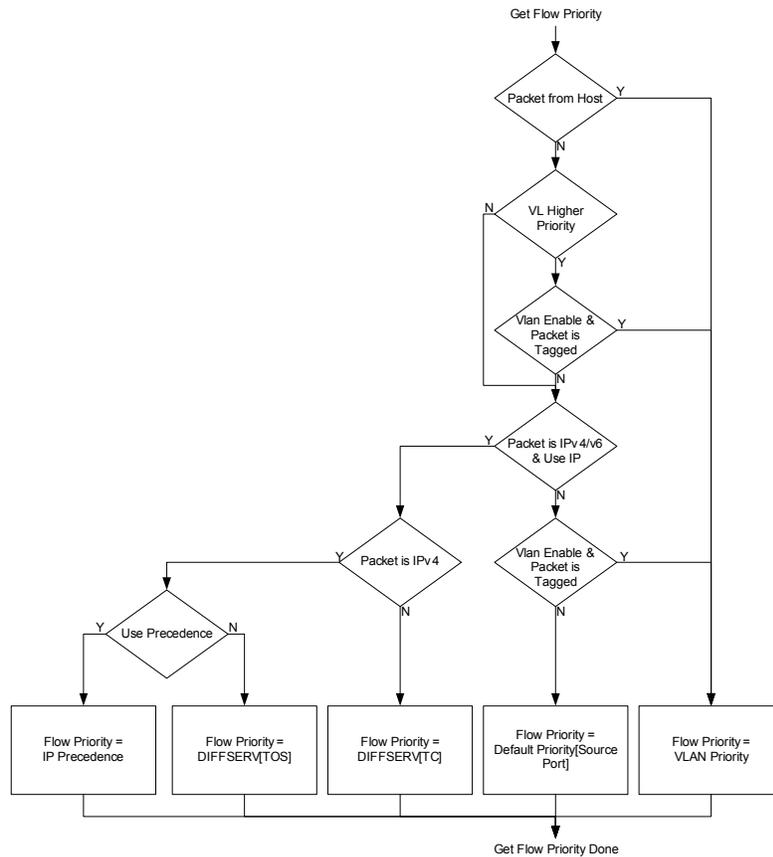
Figure 6.8 Switch Engine Ingress Flow Priority Calculation
