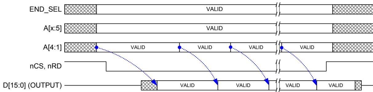
**Figure 8.4 Functional Timing for PIO Burst Read Operation**
