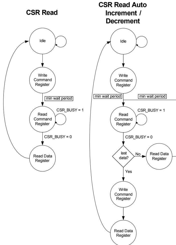
**Figure 6.2 Switch Fabric CSR Read Access Flow Diagram**
