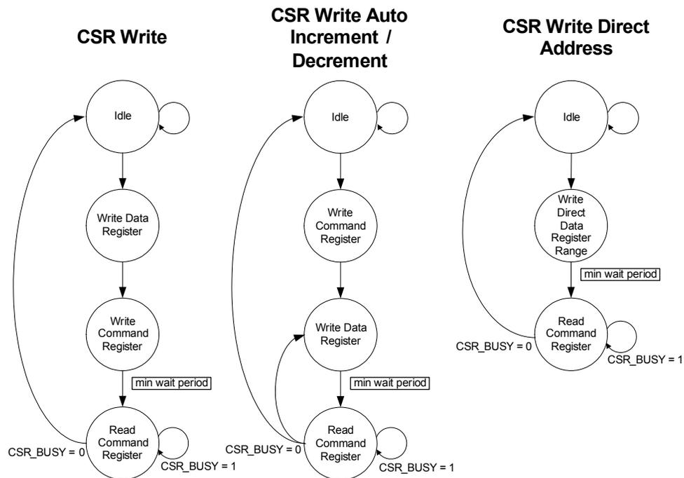
Figure 6.1 Switch Fabric CSR Write Access Flow Diagram
