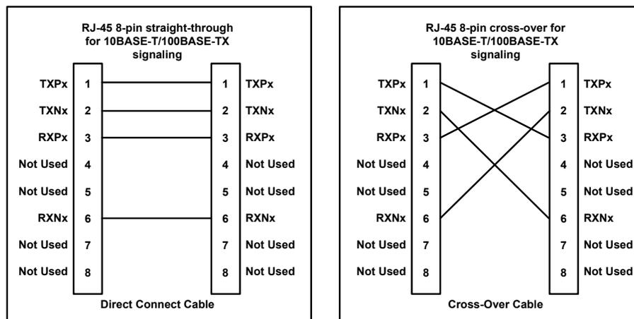
Figure 7.4 Direct Cable Connection vs. Cross-Over Cable Connection
