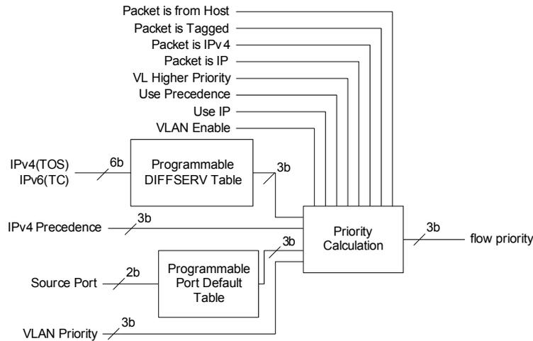
Figure 6.7 Switch Engine Ingress Flow Priority Selection
