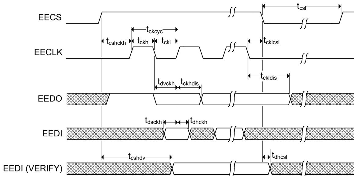
Figure 15.10 Microwire Timing
