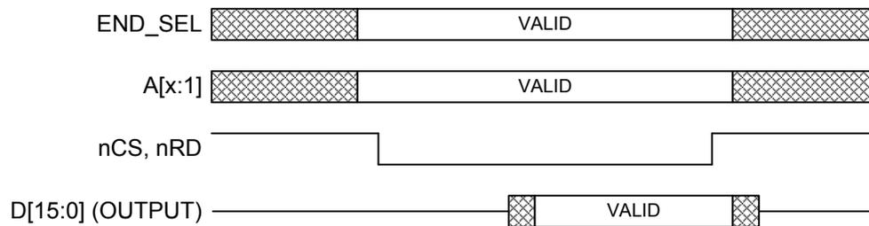
**Figure 8.3 Functional Timing for PIO Read Operation**
