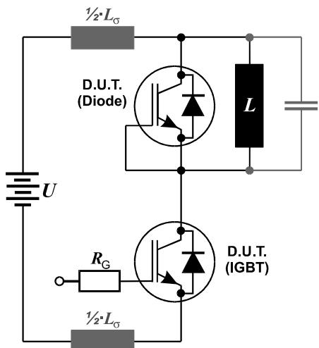
**Figure E. Dynamic test circuit**
