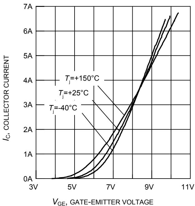
**Figure 7. Typical transfer characteristics**
