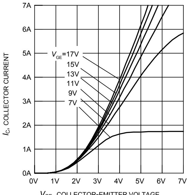
**Figure 5. Typical output characteristics**
