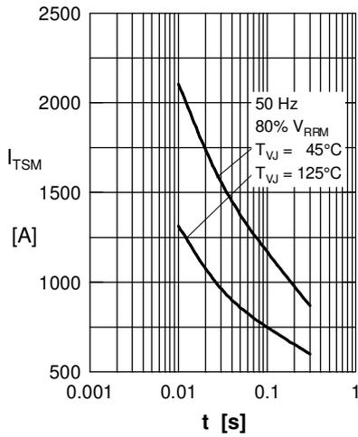
Fig. 1 Surge overload current  $I_{TSM}$ ,
