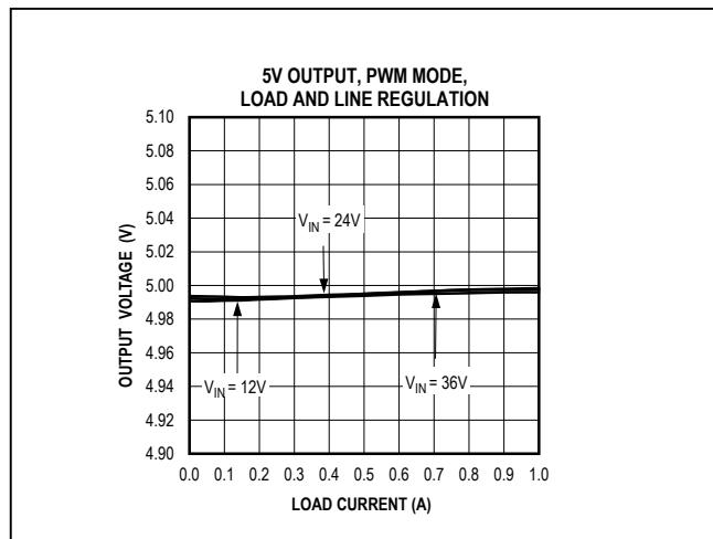
Figure 1. MAX17542G 5V Output Load and Line Regulation
