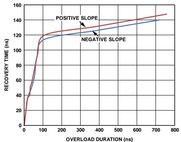
Figure 36. Output Overload Recovery Time vs. Overload Duration
