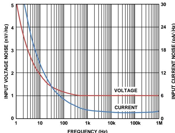
Figure 3. Input Voltage and Current Noise vs. Frequency
