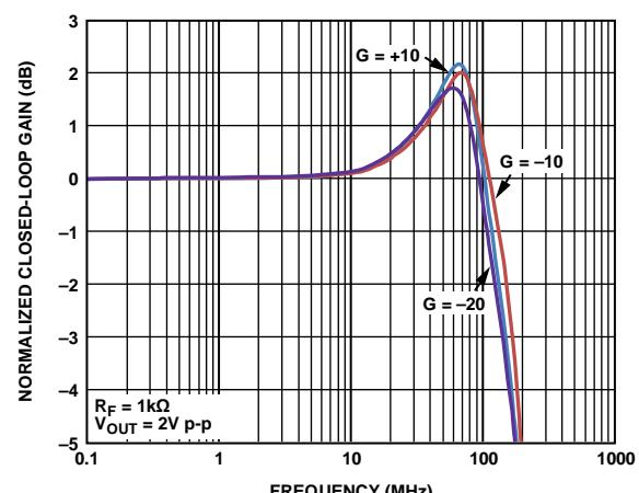
Figure 12. Large Signal Frequency Response vs. Gain
