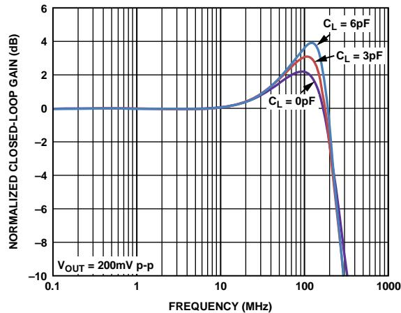
Figure 15. Small Signal Frequency Response vs. Capacitive Load
