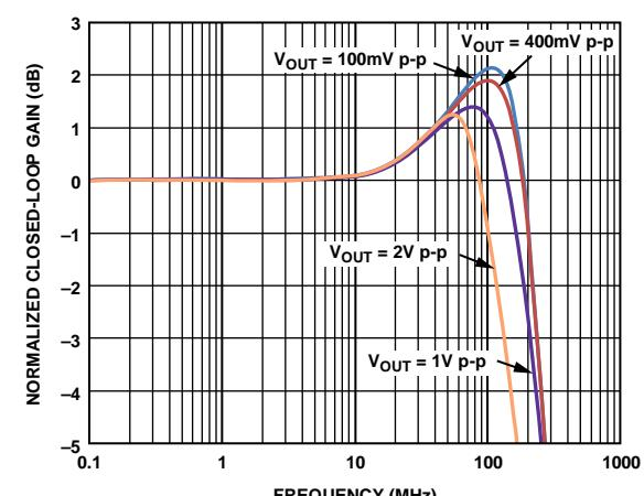
Figure 13. Frequency Response for Various Output Voltages
