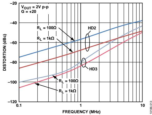
Figure 20. Harmonic Distortion vs. Frequency,  $G = +20$
