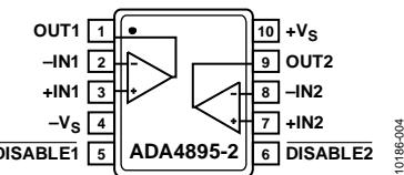
Figure 7. 10-Lead MSOP Pin Configuration for the ADA4895-2
