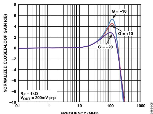
Figure 9. Small Signal Frequency Response vs. Gain
