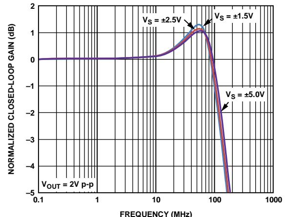
Figure 11. Large Signal Frequency Response vs. Supply Voltage
