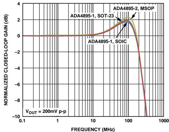
Figure 14. Small Signal Frequency Response vs. Package
