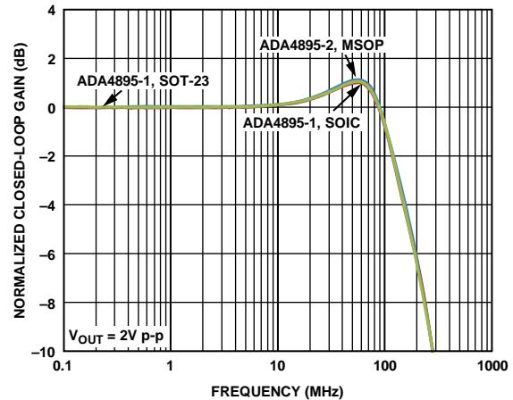
Figure 17. Large Signal Frequency Response vs. Package
