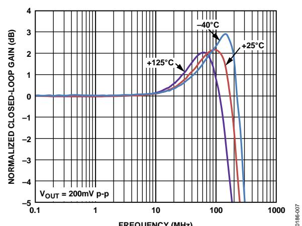
Figure 10. Small Signal Frequency Response vs. Temperature
