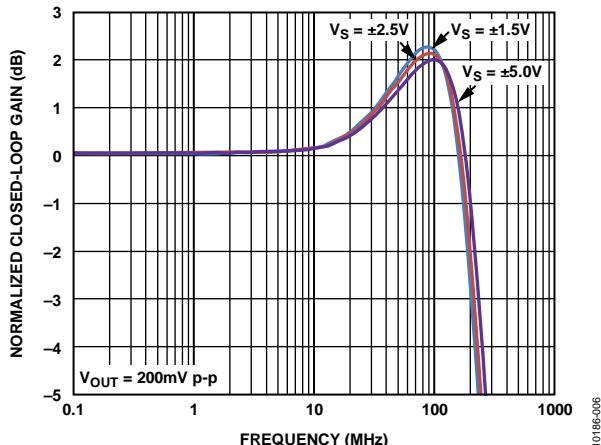
Figure 8. Small Signal Frequency Response vs. Supply Voltage
