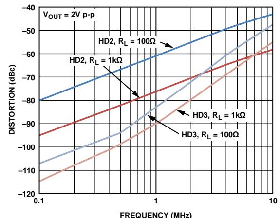
Figure 16. Harmonic Distortion vs. Frequency for Various Loads
