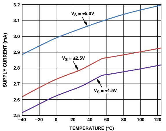
Figure 34. Supply Current vs. Temperature for Various Supplies
