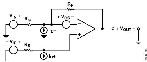
Figure 46. Typical Connection Diagram and DC Error Sources
