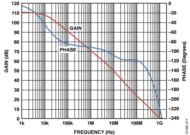
Figure 18. Open-Loop Gain and Phase vs. Frequency
