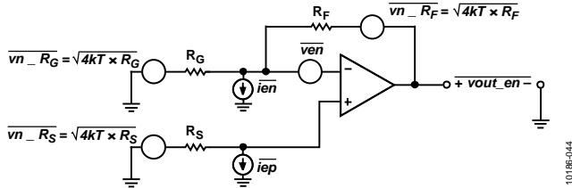
Figure 48. Noise Sources in Typical Gain Configurations
