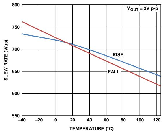
Figure 33. Slew Rate vs. Temperature
