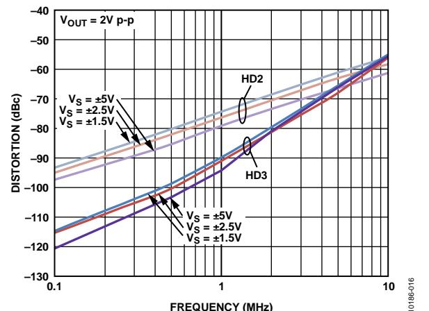
Figure 19. Harmonic Distortion vs. Frequency for Various Supplies
