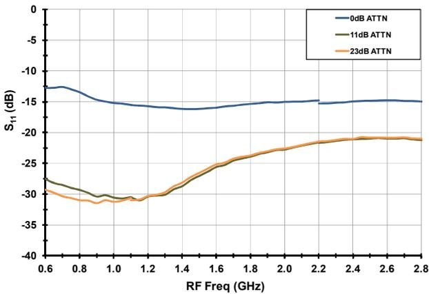
**S22 (device+C5 cap) [T<sub>AMB</sub> = 25C, V<sub>CC</sub> = 5.00 Volts]**
