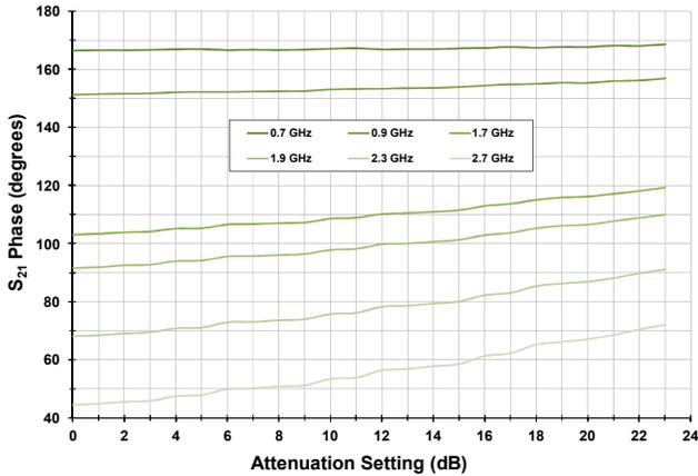
**S21 (device+C5 cap) [T<sub>AMB</sub> = 25C, V<sub>CC</sub> = 5.00 Volts]**
