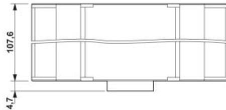
The dimensional drawing shows the item along with the lower part of the housing (terminal installation depth 11.1 mm) and the housing cover
