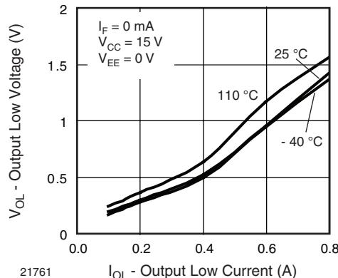
Fig. 13 - Output Low Voltage vs. Output Low Current
