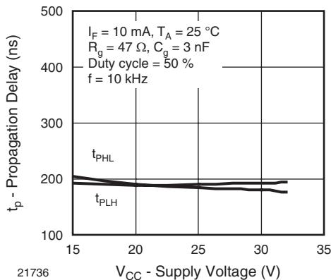
Fig. 19 - Propagation Delay vs. Supply Voltage
