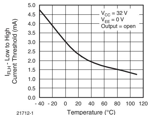
Fig. 17 - Low to High Current Threshold vs. Temperature
