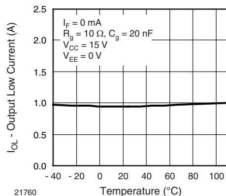
Fig. 12 - Output Low Current vs. Temperature
