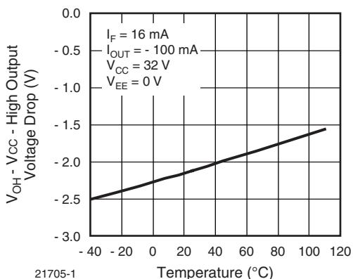
Fig. 9 - High Output Voltage Drop vs. Temperature
