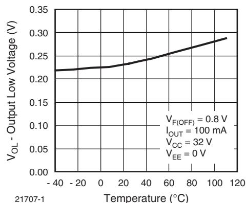
Fig. 11 - Output Low Voltage vs. Temperature
