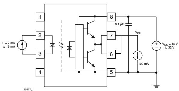
Fig. 3 -  $V_{OH}$  Test Circuit
