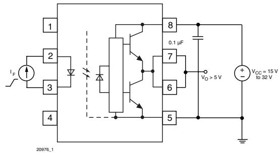
Fig. 5 -  $I_{FLH}$  Test Circuit
