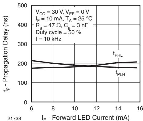
Fig. 21 - Propagation Delay vs. Forward LED Current
