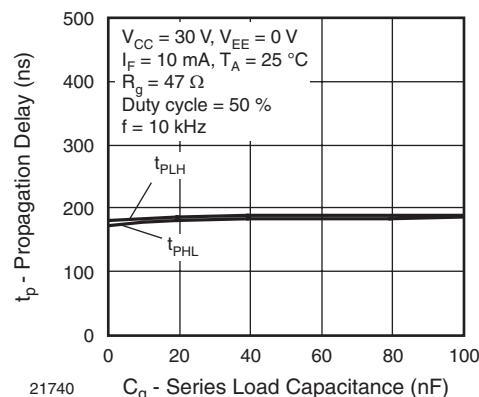
Fig. 23 - Propagation Delay vs. Series Load Capacitance
