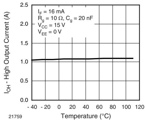
Fig. 10 - High Output Current vs. Temperature
