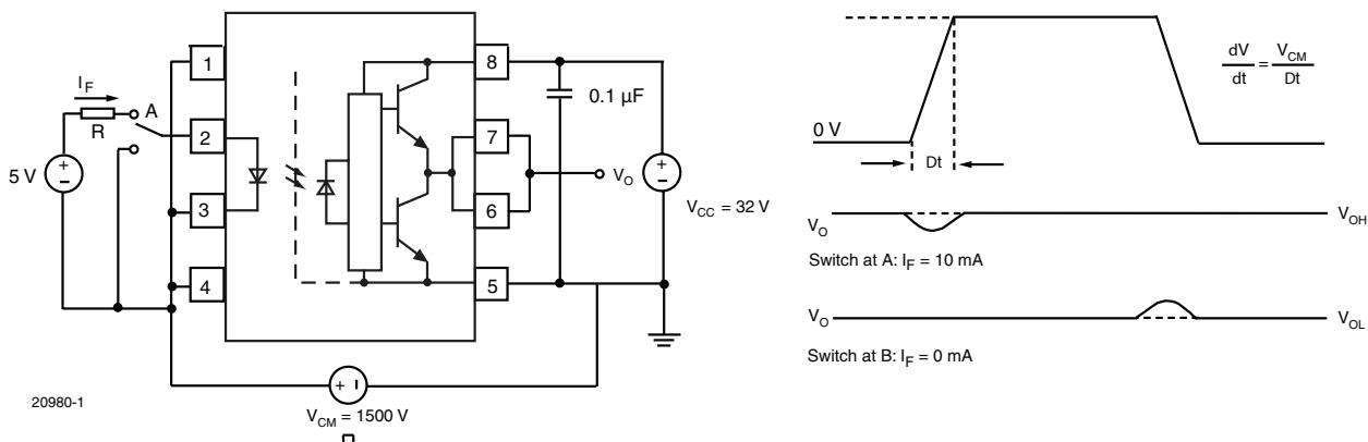
Fig. 8 - CMR Test Circuit and Waveforms
