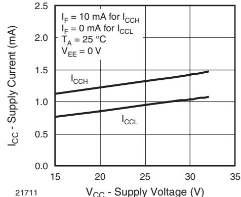
Fig. 16 - Supply Current vs. Supply Voltage
