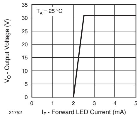
Fig. 18 - Transfer Characteristics
