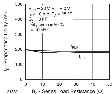
Fig. 22 - Propagation Delay vs. Series Load Resistance
